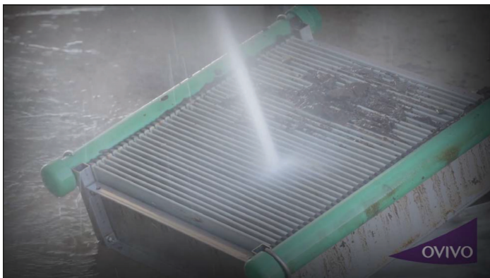
Power washing sludge off Ovivo's silicon carbide membrane used to thicken sludge without polymer that can be retrofit into existing tanks to achieve Class B stabilization.
