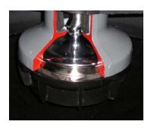
head conditions. The large inlet grinder operates at slower speeds and draws material into the pump stator (see photo)
