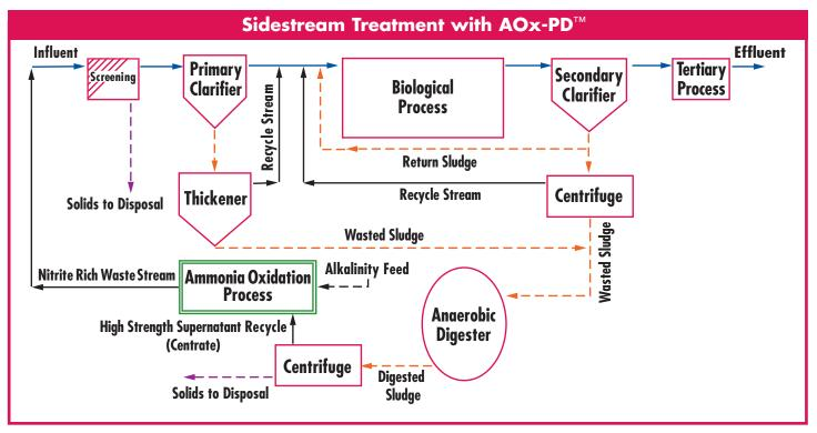
Although some denitrification occurs within the bioreactor, AOx-PD<sup>™</sup> takes advantage of the environmental conditions within the influent piping system and headworks of a typical municipal wastewater treatment plant by introducing the partially treated (high nitrite concentration) recycle stream into the collection system. Therefore, the collection system and headworks are utilized as a denitrification reactor.
