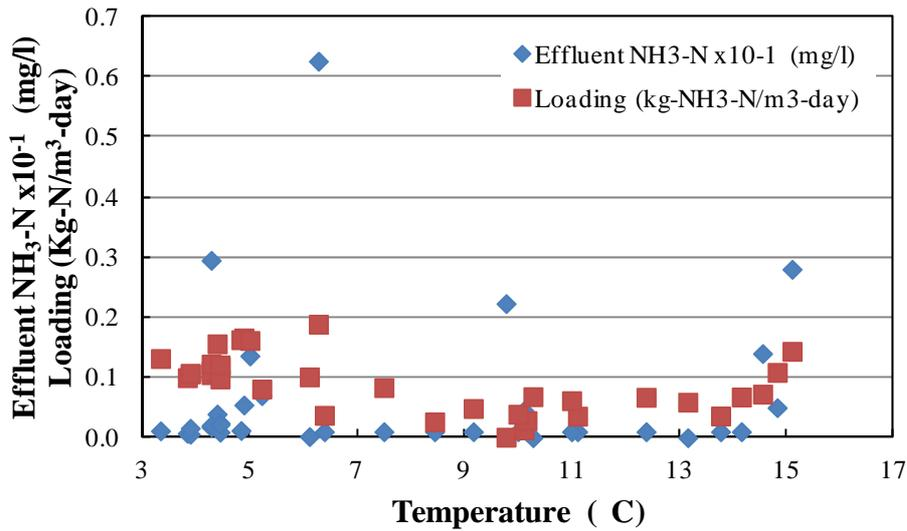
**Figure 2.** Ammonia Loading and Effluent Concentration versus Temperature
