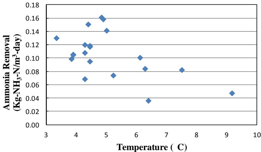
**Figure 3.** Ammonia Removal versus Temperature
