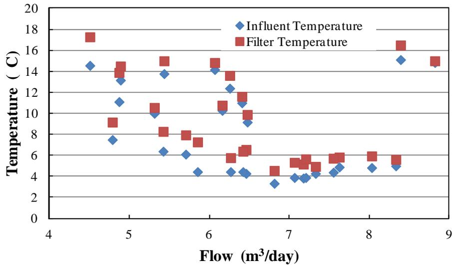
**Figure 4.** Influent and Filter Wastewater Temperature versus Flow
