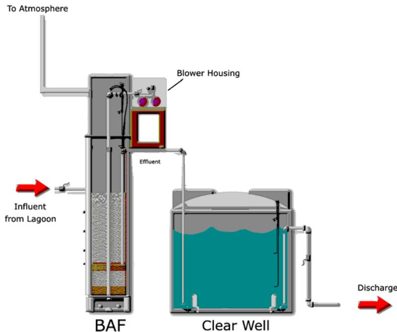
**Figure 1.** Pilot Plant Operated at the Waverly Township Facility
