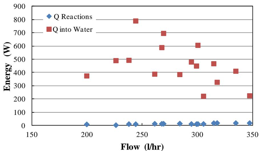
**Figure 6.** Energy from Reactions and Energy Required to Heat the Water versus Flow
