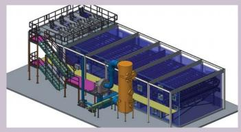
The low temperature nature of the thermal sludge dryer enables the BioCon<sup>™</sup> dryer to utilize various thermal energy sources including thermal oil, air or steam. Thermal efficiency can be further increased by employing BioCon<sup>™</sup> Energy Exchange System. Fuel sources for the Biocon<sup>™</sup> system include natural gas, biogas, or fuel oil.
