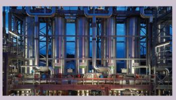
Veolia's patented thermal hydrolysis technologies are considered the next generation high solids thermal hydrolysis processes as they are able to process sludge directly from dewatering units, without any dilution (proven operation from 22% DS up to 32% DS in real world use), using the state-of-art dynamic mixers to instantaneously condense steam on to sludge.
