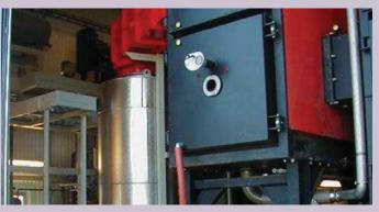
Additionally, the BioCon<sup>™</sup> dryer can be fueled by the biosolids end product by incorporating the ERS which can result in an autogenous system by combusting the end product and utilizing the heat of combustion to fuel the dryer.
