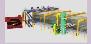
**BioCon™ ERS** (Energy Recovery System) is a safe and sustainable drying and combustion system that combines the efficiencies of a convective air low temperature belt dryer with a biomass furnace to recover sensible heat and combust all organic material, including PFAS compounds.
